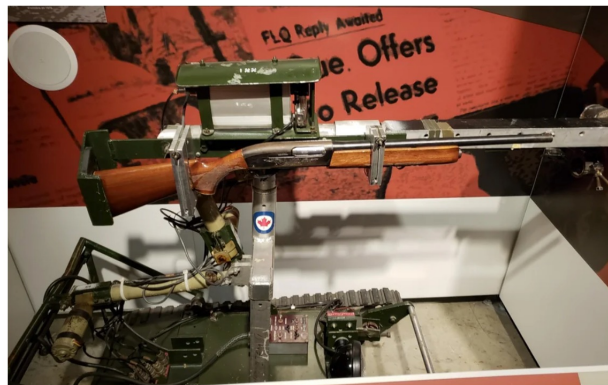
This "robot" was neither autonomous nor especially sophisticated. It was used by the Canadian Armed Forces for bomb disposal during the 1970 FLQ Crisis. Canadian War Museum collection.
